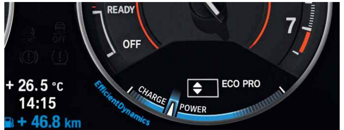
ECO PRO Mode. Driving in ECO PRO Mode helps customers achieve fuel savings of up to 20 percent, depending on their individual style of driving. This mode optimises accelerator and transmission response as well as shift points, and intelligently adapts the heating/air conditioning strategy. ECO PRO tips help the driver drive even more efficiently. The bonus range shown by the on-board computer indicates how many additional miles the driver has gained, thanks to the increased efficiency in ECO PRO Mode since the last fill-up.
