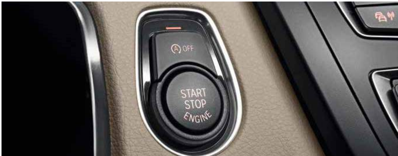
The Auto Start/Stop Function switches off the engine when the vehicle comes to a temporary standstill (e.g. at traffic lights) to further reduce overall fuel consumption.
