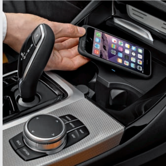
Telephony with wireless charging 1 offers a comprehensive telephony package with Bluetooth connectivity.
