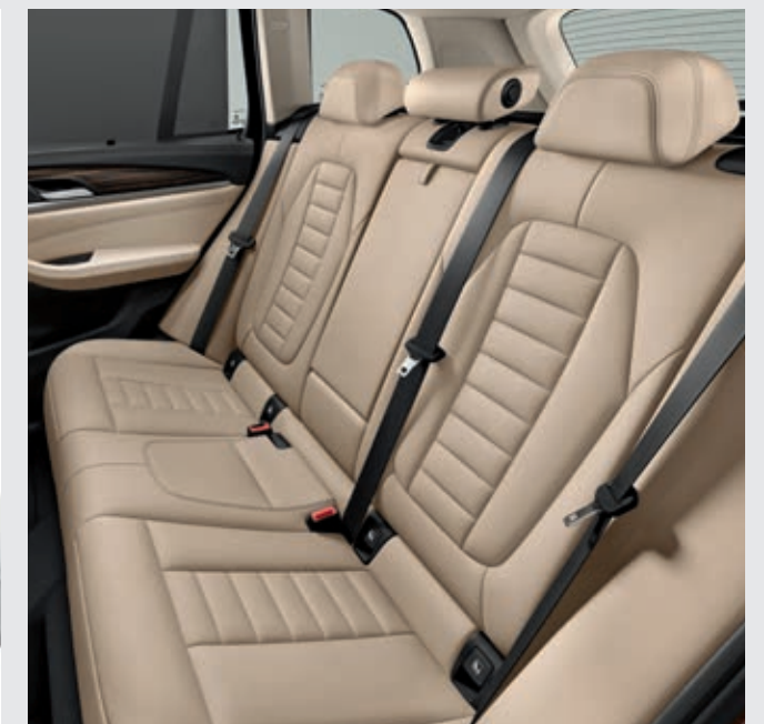
Rear seat backrests divisible in a 40:20:40 ratio ensuring flexibility when transporting people, luggage and other various items.
